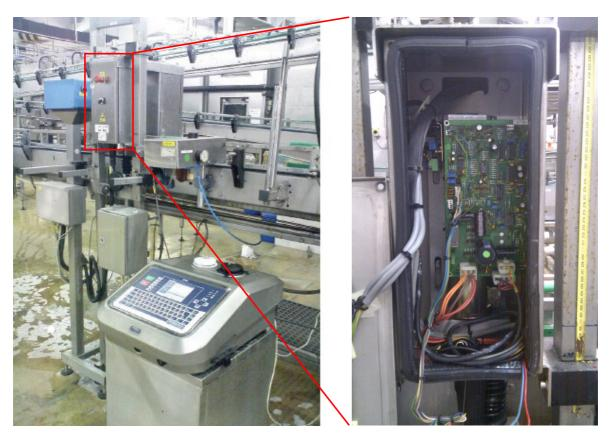
Photographs: the original gauging system on the can filling line (left), and inside the gauge cabinet (right): the X-ray tube is mounted on the rear of the circuit board.
