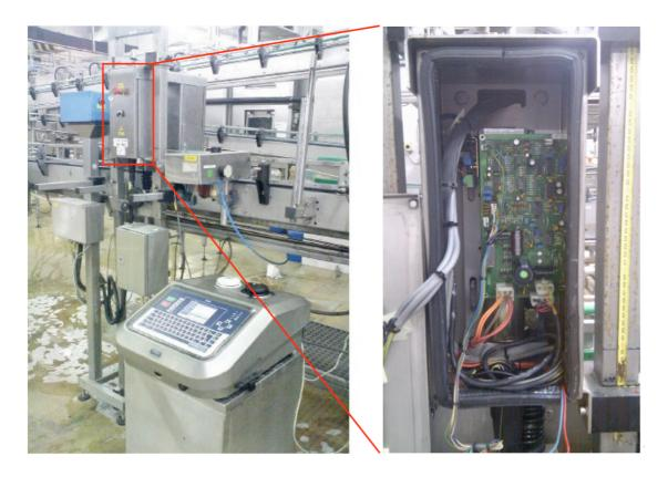
Figure 1 – The original gauging system on the can filling line (left), and inside the gauge cabinet (right): the X-ray tube is mounted on the rear of the circuit board.
