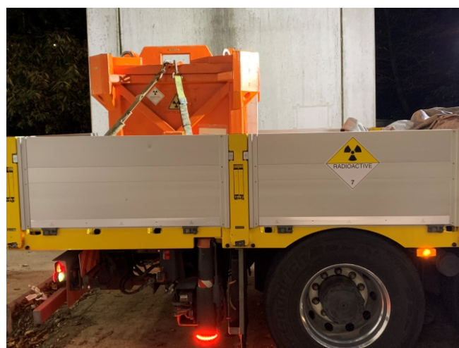
Figure 2. Hazardous goods transporter with the resistant transport box in which the source container is placed using a crane.
