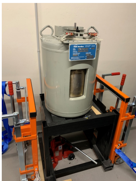
Figure 1. Lead source container with a high activity Cs-137 source from a blood irradiator. The silver opening was used to place the blood in the irradiation cell (the electronics and housing of the blood irradiation device have already been removed).
