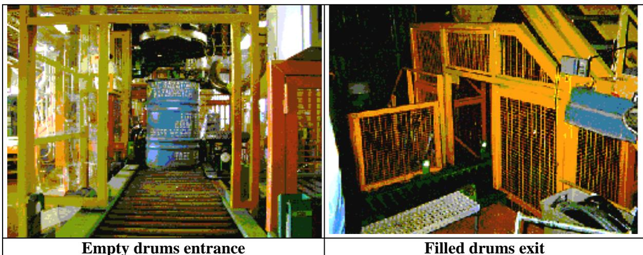
Figure 4: Openings in the filling station confinement
