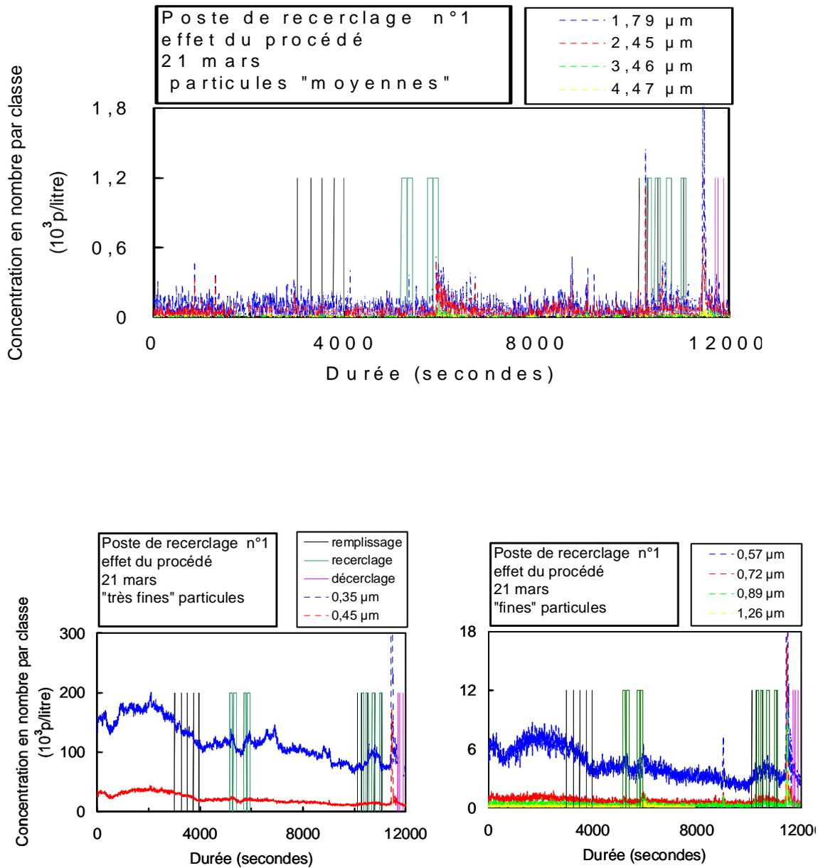
Figure 11: Particles concentration at the rebanding station (GRIMM, March 21). Medium particles above, fine and ultra-fine particles below.
