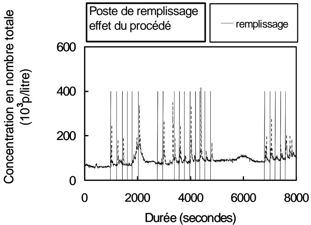
**Figure 8: Particles concentration at the filling station (GRIMM, March 19). Fine particles above, all particles below.**
