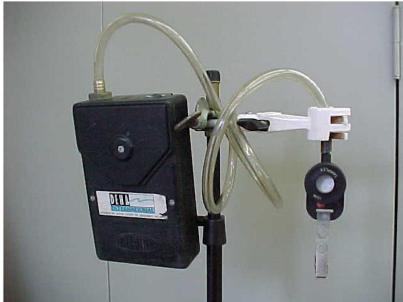
**Figure 3. Air pump and IOM filter holder with filter**
