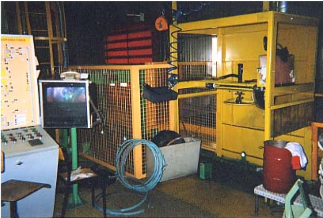
**Figure 12 : New dynamically confined rebanding workstation, equipped with a lid shutting device**
