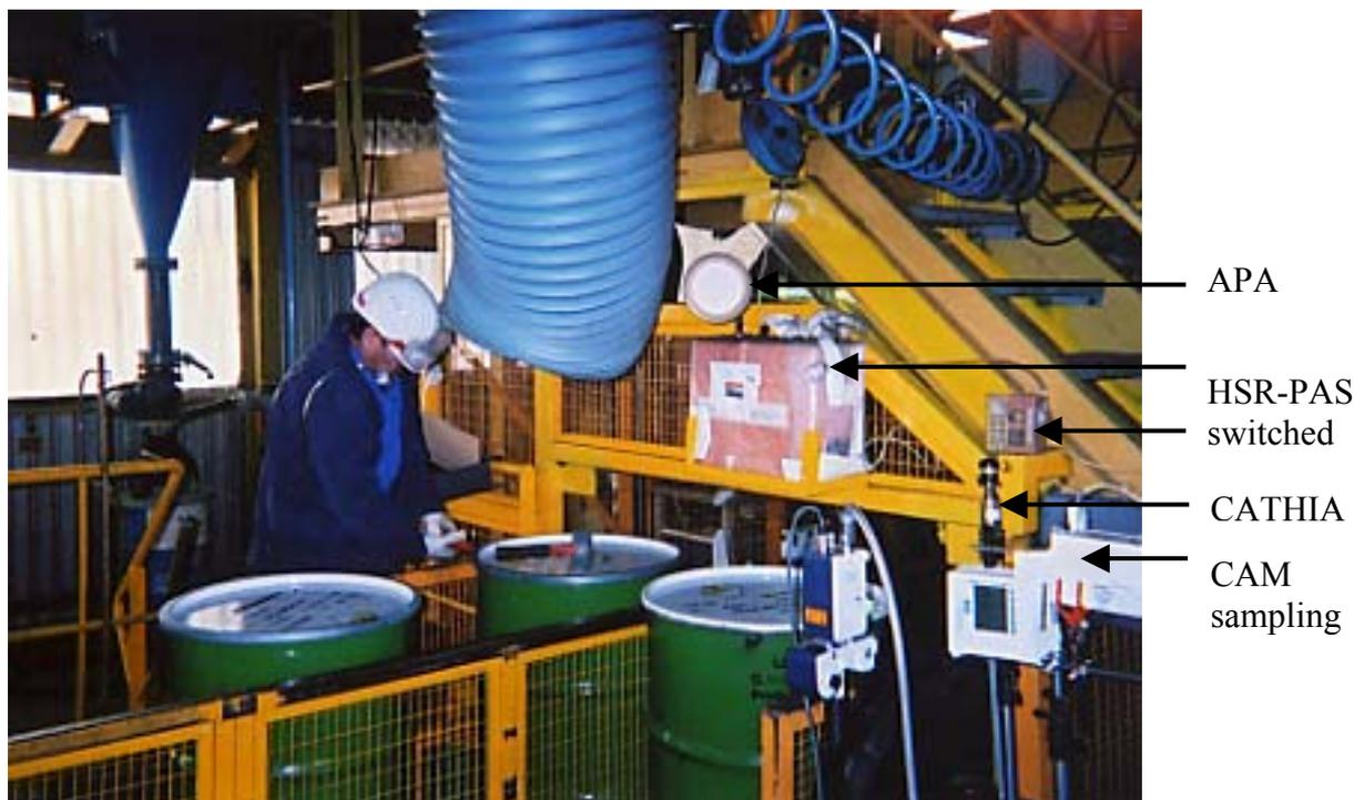
**Figure 5: Detailed measurements with FAS, PAS, switched PAS, CAM and RTMD**
