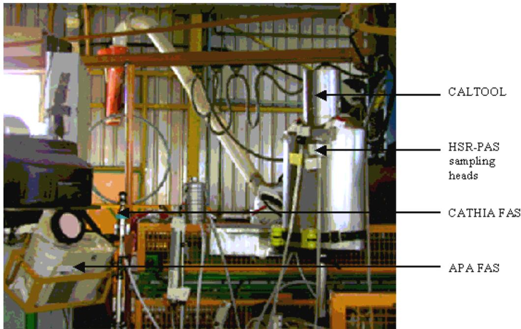
**Figure 7: On-site comparison of air samplers with reference air sampling devices**
