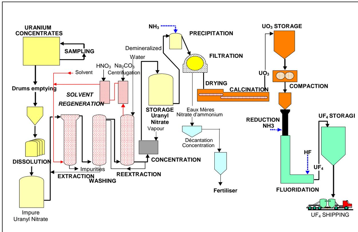
**Figure 1 : Wet Process for refining/conversion of uranium mining concentrates**
