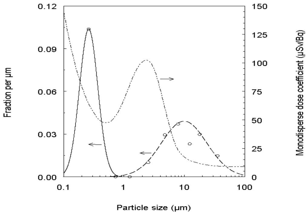
**Figure 5. Particle size distribution of generated phosphorus slag dust relative to total dust.**
