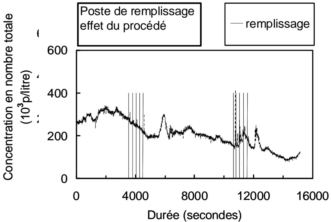
Figure 9: Particles concentration at the filling station (GRIMM, March 21). Fine particles above, all particles below.
