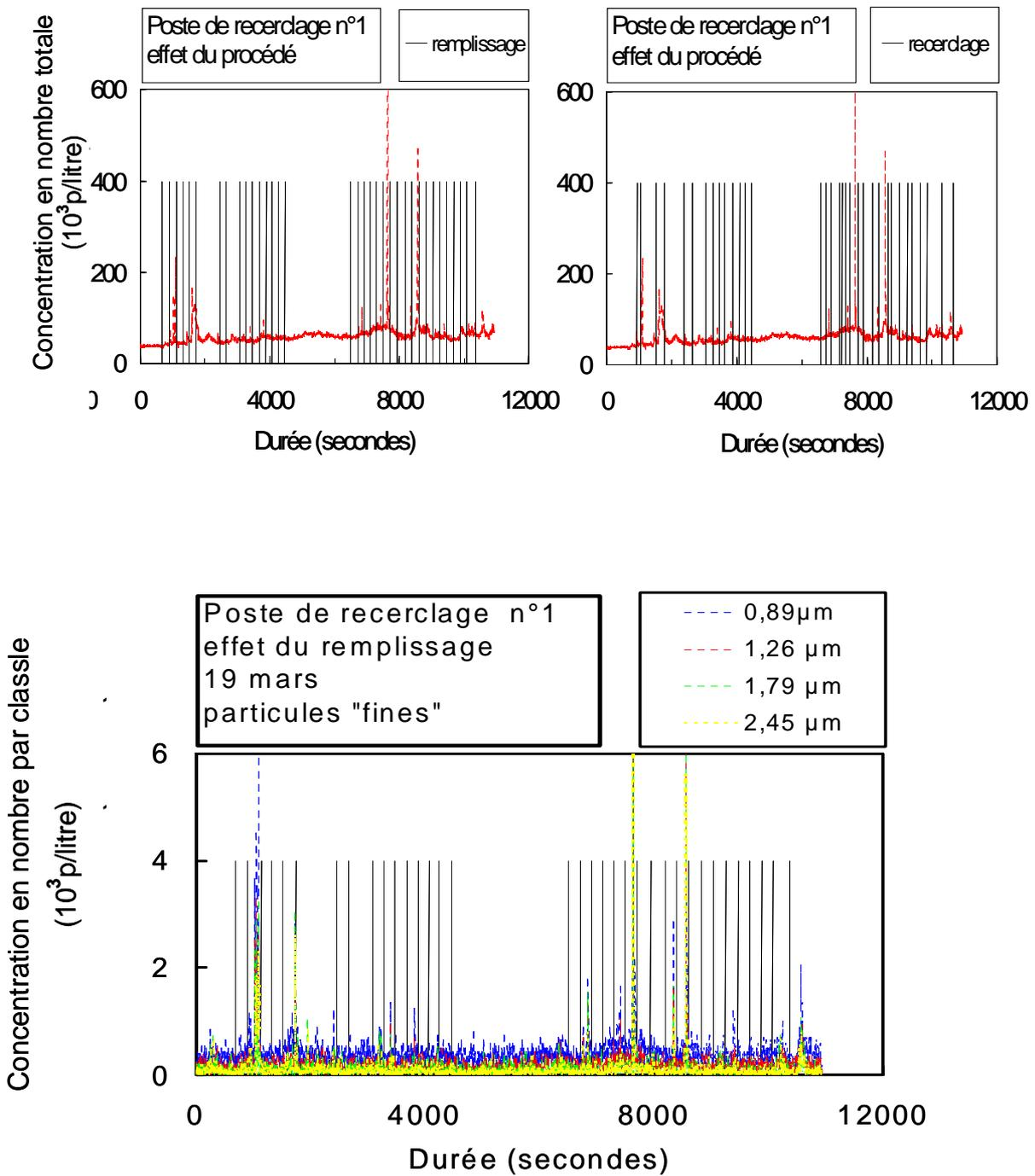
Figure 10: Particles concentration at the rebanding station (GRIMM, March 19). All particles above, fine particles below
