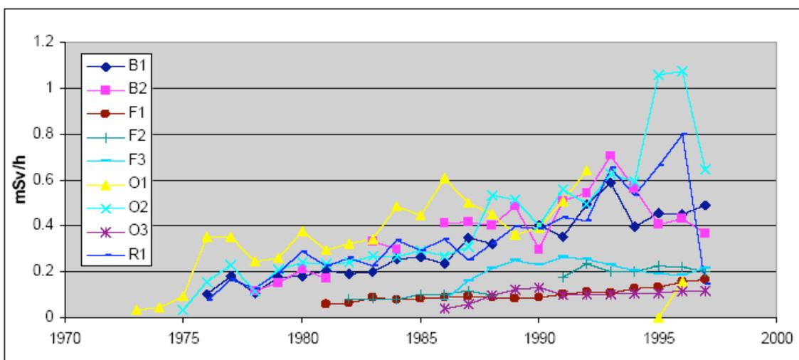
Figure 2: Recorded radiation levels (mSv/h) near cooling systems at Swedish Boiling Water Reactors between 1973- 1997.
