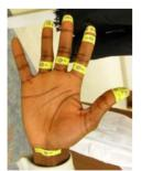
*Figure 1. Standard measuring positions (additional: detectors on the nails of index, middle and ring finger)*
