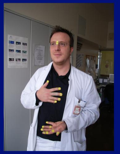
Thin-layer thermoluminescence detectors (TLD)
