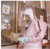
Decontamination of a laboratory hood
